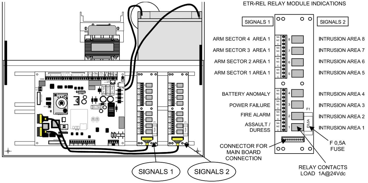
NOTE: USE NYLON CLIPS SUPPLIED TO MOUNT ETR-REL MODULE. FIX THEM AS INDICATED USING SOME OF THE HOLES (5) AVAILABLE ON MODULES AND METAL SUPPORTS BENEATH.
