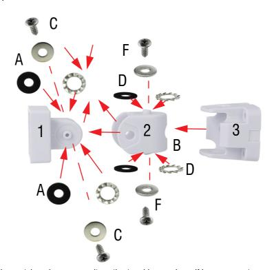
**Notes:** in the mounting kit are also provided four self-locking metal washers, <u>as an alternative to rubber washers</u>, if is necessary to block stronger the joint.
