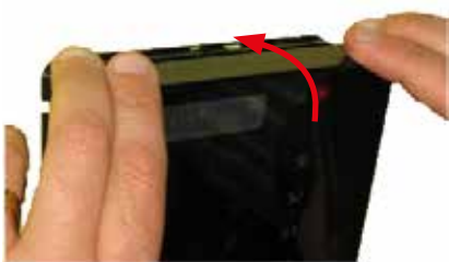
To close the keypad, hook the lower part to the upper one.
