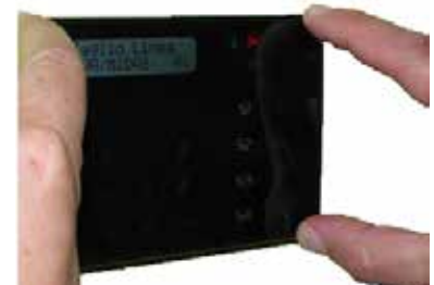
Gently press on both the sides until the keypad is fastened to the base.
