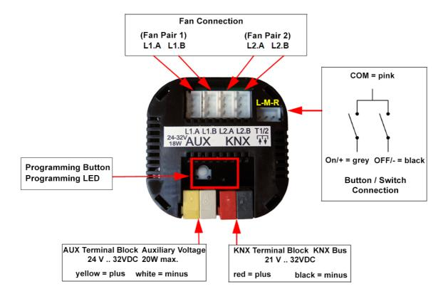
The KNX clamp is connected to the KNX bus via the supplied terminal block (red (+) / black (GND)). The auxiliary voltage is connected via the supplied terminal block (yellow (+) / white (GND)). The fans are mounted according to the lunos specification and connected via the supplied preceded connector. Optionally, potential-free button / switch can be connected via the supplied connector.
