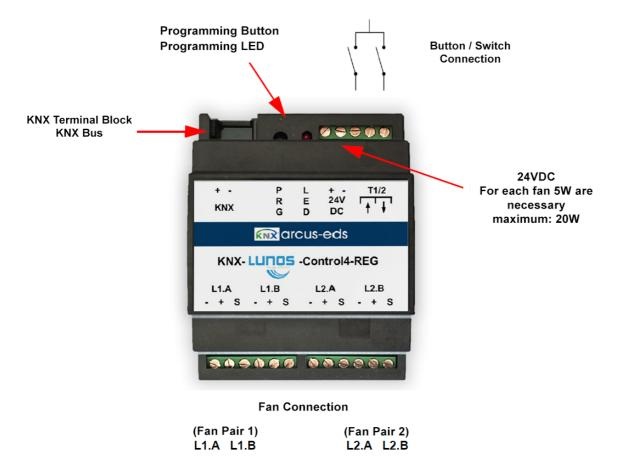
The KNX clamp is connected to the KNX bus via the supplied terminal block (red (+) / black (GND)). The auxiliary voltage is connected via a screw clamp. The fans are mounted according to the lunos specification and connected via the screw terminals. Optionally, potential-free button / switch can also be connected via screw terminals.
