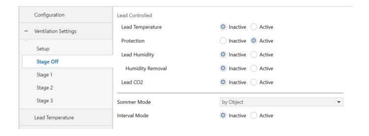
Functional block fan stage operating modes - Parameters
