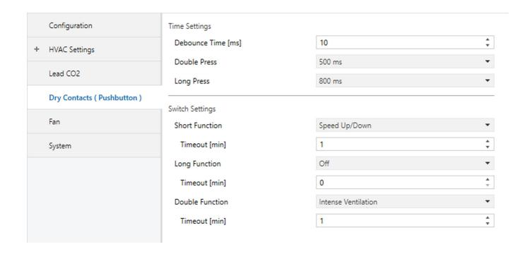
Functional block potential free contacts (Push buttons) - Parameters
