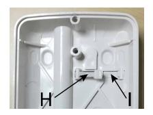
In case of corner installation, in order to ensure protection from removal from the mounting surface, it will be necessary to move the H lever (which operates the corresponding micro-switch at the back of the board) to the position of the plastic plug I that closes the detector angle.
