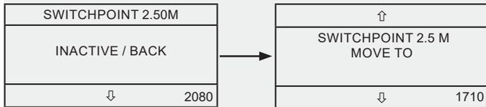
Enable / move to the desired position using ↑↓
