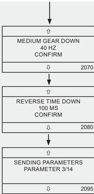
Select the frequency for the desired speed via ↑↓
