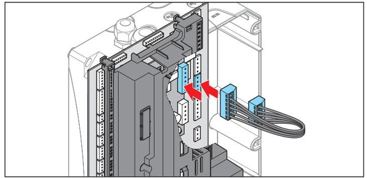
6. Connect the control unit and the induction loop module with the connection cable
