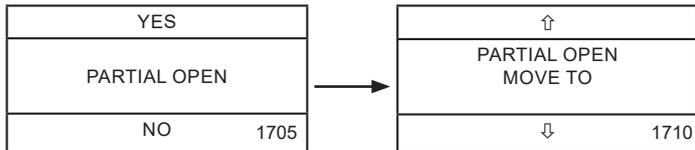
Move to the desired partial opening height via ↑↓
