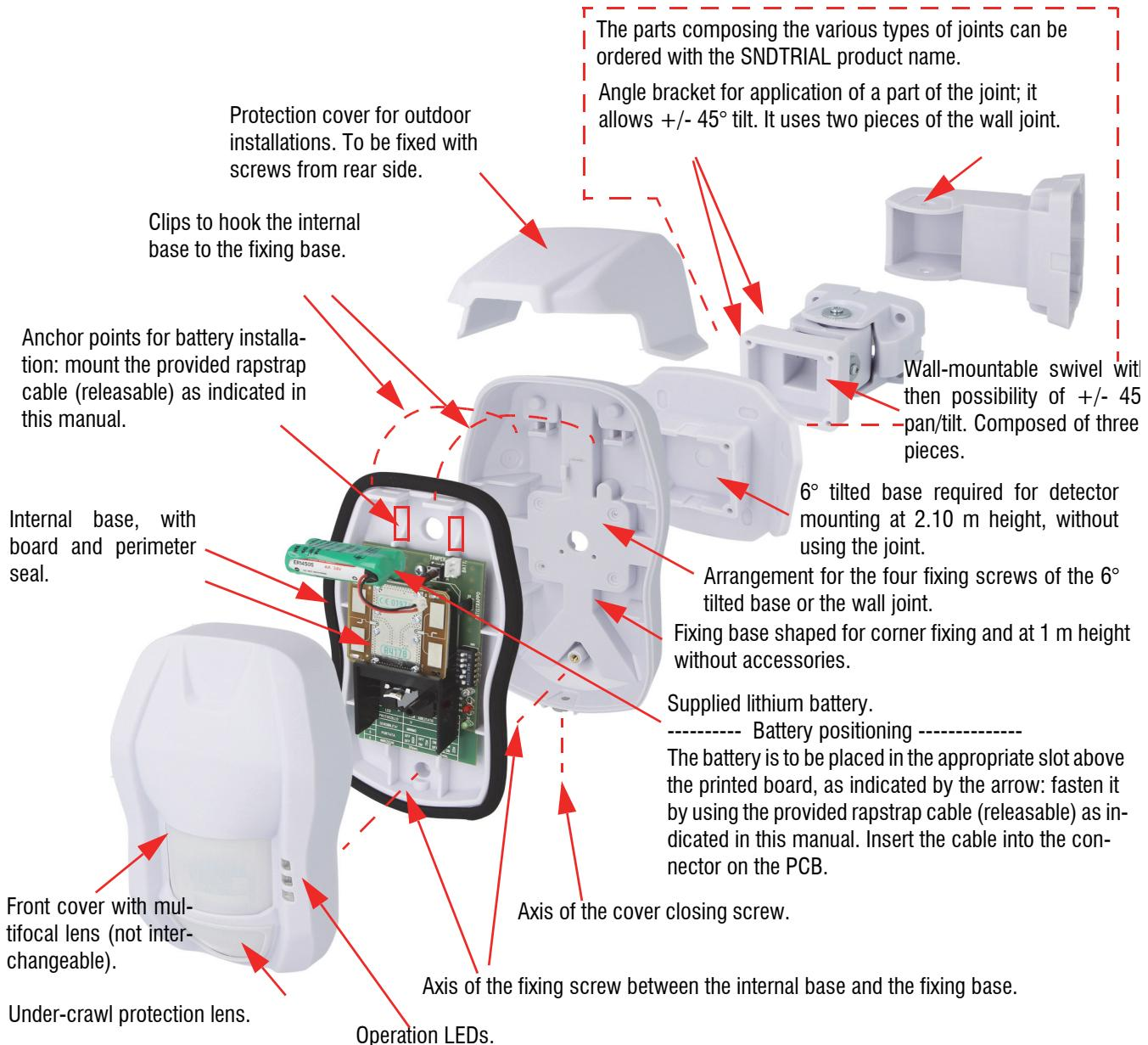
**Note:** the joints are supplied with the **SNDTRIAL** product, they are to be mounted according to the needs and they are equipped with rubber washers with special clutch function. For the assembly see the specific data sheet.
