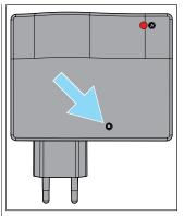
Press and hold the Reset button using a thin (but not sharp) object until the Status LED blinks red
