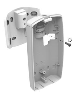
fix the base to the bracket using the suitable screw (D) With optional joint:
