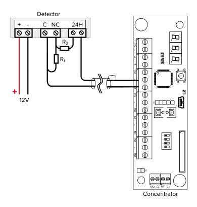
wire concentrator zones, according to the set balancing mode (see paragraph 5.2 p. 5)
