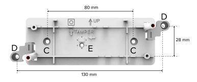
install the base on the mounting surface with screws and inserts using central holes (C) or side hinges holes (D)
