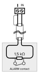
Fast zone management requires setting type 1 balancing (R.  $= 1500 \Omega$ , R<sub>2</sub>  $= 1500 \Omega$ ).
