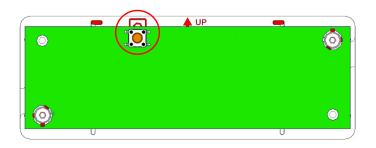
Make sure the switch for protection against opening (on board top) is on the upper side as indicated by the symbol on case base.
