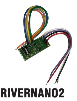
Miniaturized serial line concentrator with 2 programmable inputs
