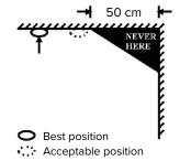
In case of installation on flat ceilings, position each detector as close to the center of the ceiling as possible. In any case, leave a distance of at least 50 cm from any wall or corner.
