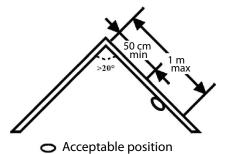
In case of installation in rooms that have sloped ceilings (slope higher than  $20^{\circ}$ ), position the detector at a distance between 0.5 m to 1 m from the ceiling peak.
