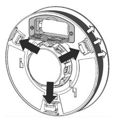
remove the detector outer cover: press one tab at a time and lift the cover on each of the three closing points
