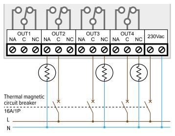
The example shows a magneto-thermal circuit breaker. In fact, it is possible that the controlled resistive loads are part of different lines and each has its circuit breaker.
