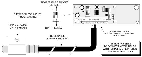
Inputs connection with gas detectors with 4-20mA interface, e.g. RGLOOP-xx.
