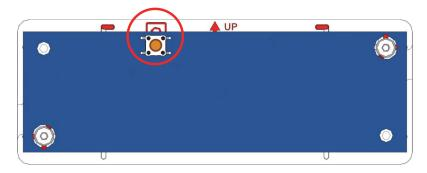
Insert the PCB on the plastic supports (the board in the picture is for reference only).
