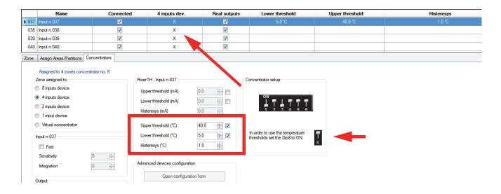
In the example is viewed a concentrator with only an input connected to the temperature probe. The thresholds are displayed such as example and, if necessary, can be enabled the below or above thresholds. The condition is normal if the detected value remains within the two thresholds; an alarm is generated if it exceeds the threshold value.
