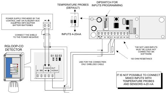
Another type of inputs connection with devices equipped with 4-20mA interface.
