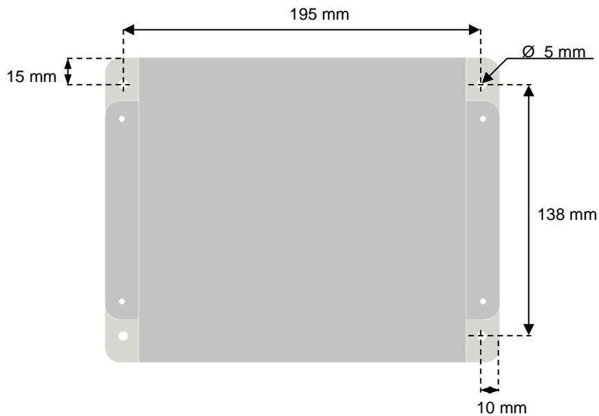
**Figure 7.3** Top view<sup>1</sup> (screw holes size)
