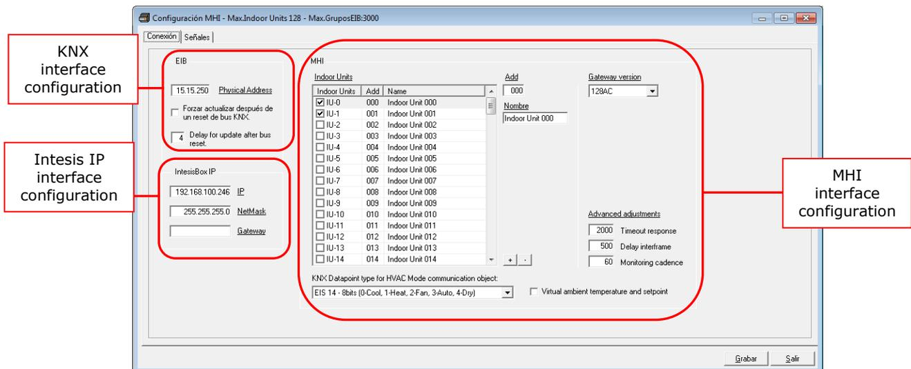
Figure 4.2 LinkBoxEIB configuration tab
