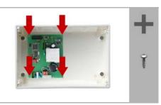
Remove the circuit board from the concealed box to be installed a keep it in a place where it is protected from dirt. It may never be exposed to dust or moisture!
