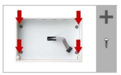
The security covering in the concealed box is attached with four screws: Loosen the screws and take off the security covering.
