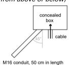
Conduit angled vertically downwards (only for cable access from above!)
