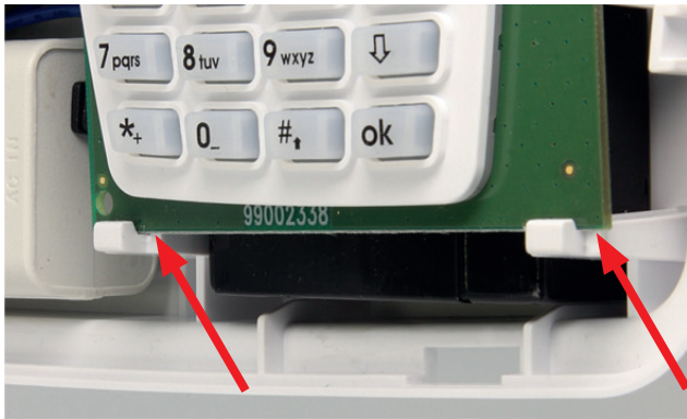
Arrange the HERCOLA main board in position on the lower holding brackets.
