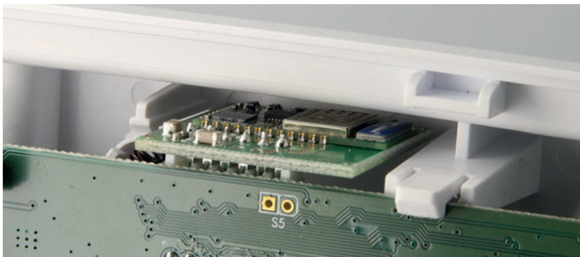
View of the HERCOLA main board with the MDWIFIH module in correct position.
