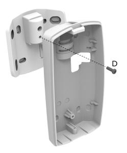
fix the base to the bracket using the suitable screw (D)
