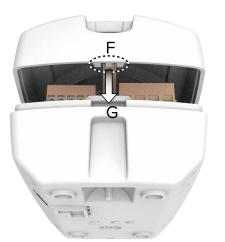
insert hooks on the upper side of the cover (F) into the base slot (G)
