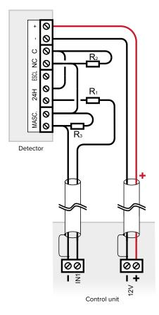
Verify the unit supports triple-balancing setup. Resitors R1 = 1000  $\Omega$ , R2 = 680  $\Omega$ , R3 = 1200  $\Omega$  are supplied with the unit.
