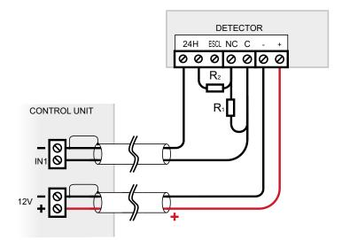
Resistors  $R1 = R2 = 1500 \Omega$  are supplied with the control unit.
