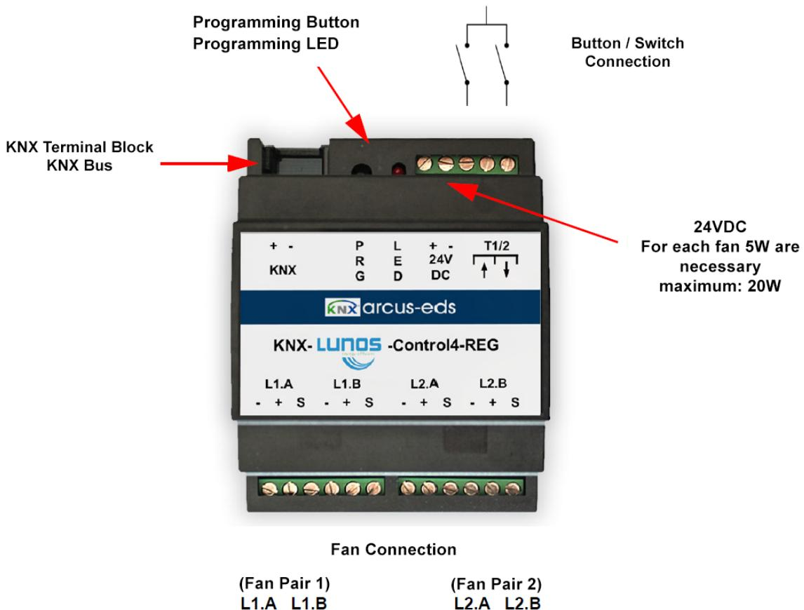
The KNX clamp is connected to the KNX bus via the supplied terminal block (red (+) / black (GND)). The auxiliary voltage is connected via a screw clamp. The fans are mounted according to the lunos specification and connected via the screw terminals. Optionally, potential-free button / switch can also be connected via screw terminals.
