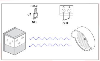
If Jumper J1 is set in position 2, when the photocell does not detect any interruption of its beam, output OUT1 is closed. For ex., if no vehicle transits between the photocell and the reflector, output OUT1 would remain closed.
