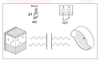
If Jumper J1 is set in position 2, when the photocell detects an interruption of its beam, OUT1 output is opened.
