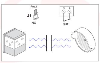
If Jumper J1 is set in position 1, when the photocell detects an interruption of its beam, output OUT1 is closed.
