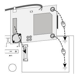
insert the spacers (supplied) in the holes on proper area on control unit board (indicated by C)
