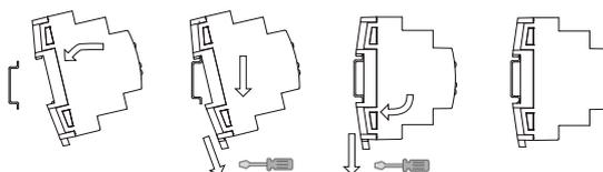
Removing DIMinBOX DX1 from DIN rail:
