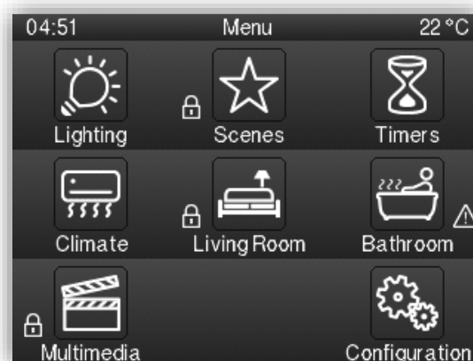
Figure 22. Menu with protection and alarms.
