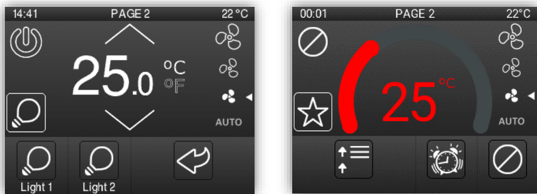
Figure 26. Thermostat + 2 boxes page / Thermostat + 2 boxes page with thermostatic Wheel.
