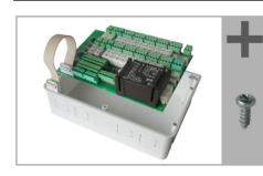
Remove the circuit board from the concealed box to be installed a keep it in a place where it is protected from dirt. It may never be exposed to dust or moisture!
