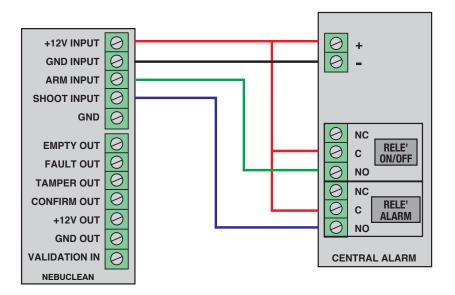
ON/OFF output of this alarm central is an open relay when the system is off and it is stably closed to positive as long as the system is turn on.
