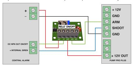
In the diagram above the control panel, as example, provides to NEBUCLEAN power supply between 11 and 14V DC 250 mA max. The ON/OFF output of this alarm is an Open Collector NPN opened when the system is off and it is stably closed to negative as long as the system turned on.
