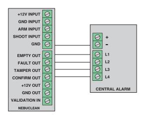
The outputs shown in the diagram are not always necessary, but only in cases where the voltage of pull-up resistance is lower than that of power supply.
