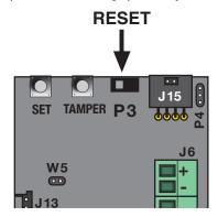
Press and release SET/RESET button on the board and check the Fault LED resets. Once done, set jumper P3 back to its starting position.
