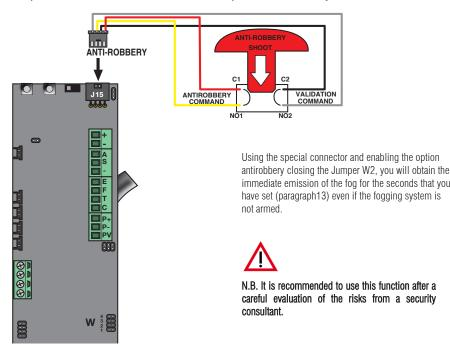
H - Example of connection of NEBUCLEAN1500 outputs with relay board.
