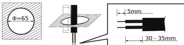
Drill a hole with  $\Phi=65\text{mm}$  on the ceiling
