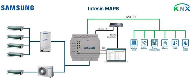
Integration of Samsung NASA's compatible systems into KNX home automation systems
