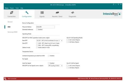
Figure 4.3 Intesis MAPS KNX configuration tab
