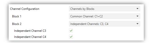
Figure 6 Channels by Blocks configuration in NarrowDIM X4.
