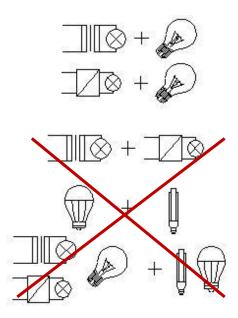
Figure 2. Combining Load Types.
