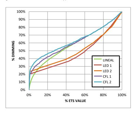
Figure 9 Dimming Patterns for LED and CFL loads.
