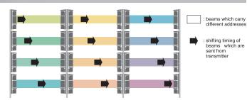
Up to 4 sets for multiple beam installation
