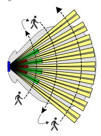
taking detector position as the point of reference, make half-circle movements from opposite directions to check coverage from both sides
