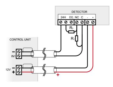
Resistors R1 = R2 = 1500  $\Omega$  are supplied with the control unit.
