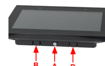
Fig. 7 To remove the display unit from the mounting unit, loosen the screw (A). Press against the lower notches (B) to release the connection. The display unit can be removed.
