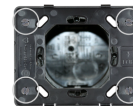
Fig. 3 If the screw domes of the box used are not covered with the mounting unit's longitudinal holes, the mounting unit can alternatively be bolted via the other holes (e.g. for other installation systems).
