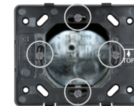
Fig. 2 Bolt the mounting unit on to the socket. The arrow („TOP“) must point upwards. Two screws (right/left or top/bottom) are enough.
