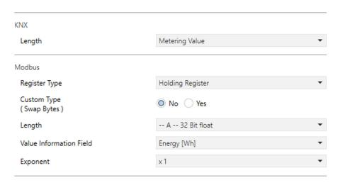
For each Modbus Channel, an object is created as input or output as well as with the parameterized data type and length.
