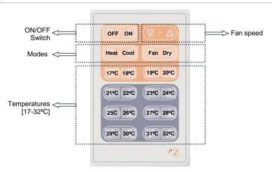
Figure 4. Testing KLIC-DI from the IR Remote
