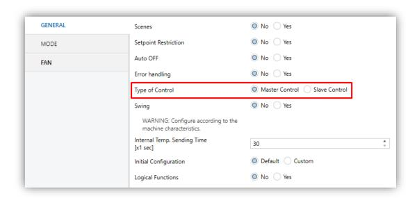
Figure 12. Configuring the type of control.
