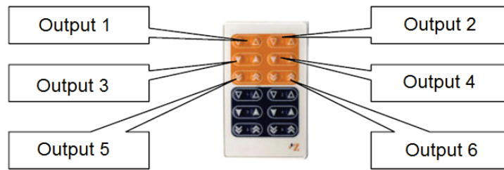
Figure 3 Controlling the outputs from the IR remote
