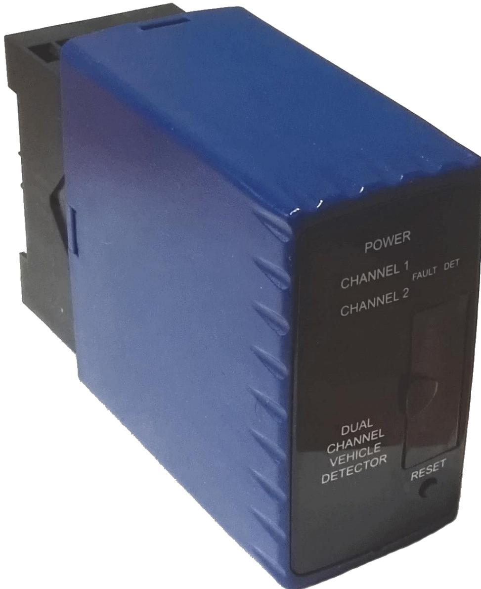
Magnetic loop sensor bi-channel 12-24
