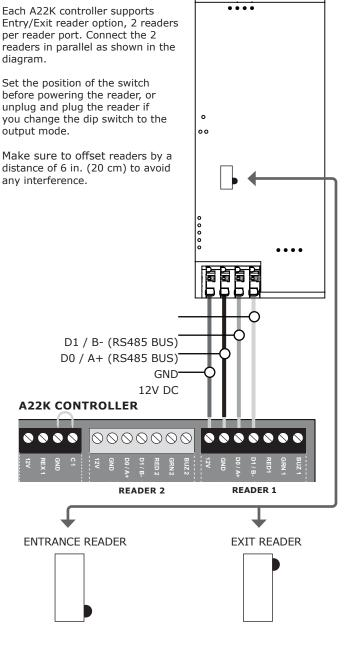
Position the switch to the bottom next to the terminal block (manufacturer setting) Position the switch to the top
