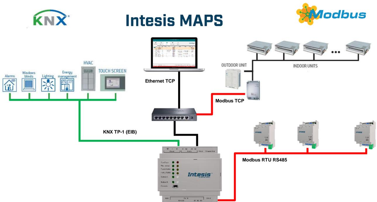
**Integration of Modbus RTU Slave or Modbus TCP Servers to KNX TP-1 (EIB)s control and monitoring systems**
