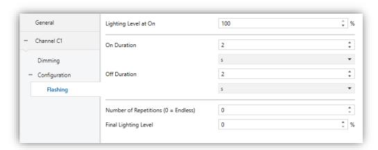
Figure 14 Flashing.
