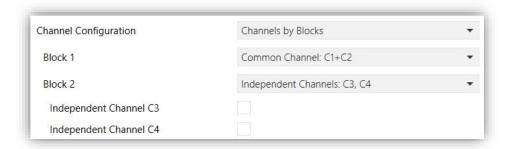
Figure 4 Channels by Blocks configuration in NarrowDIM X4.
