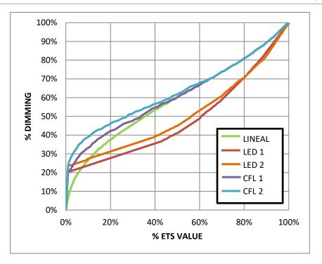
Figure 8 Dimming Patterns for LED and CFL loads.
