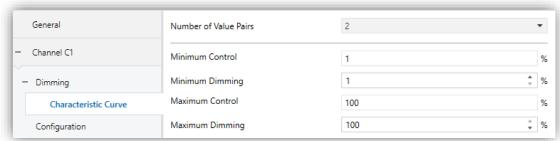
Figure 9 Characteristic Curve.
