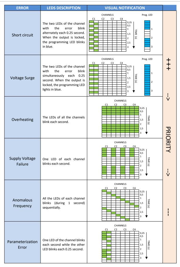
Table 2 Error Notification through the on-board LEDs.
