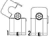
▲ Important: Secondary side cables must be connected to KES Plus (keeping polarity) <u>before</u> closing the clamp to the primary side cable.
