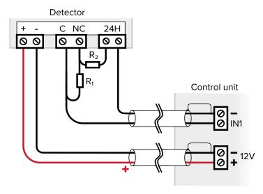
Resistors R1 = R2 = 1500  $\Omega$  are supplied with the control unit.
