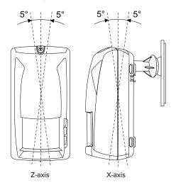
If the detector is rotated by 5 degrees compared to its initial position, 24H relay will enter the alarm condition for 5 s and red LED will start blinking slowly.
