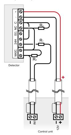
Verify the unit supports triple-balancing setup. Resitors R1 = 1000  $\Omega$ , R2 = 680  $\Omega$ , R3 = 1200  $\Omega$  are supplied with the unit.
