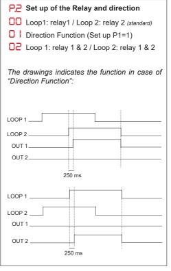
In this case the exit OUT1is connected to the START while OUT2 with the CLOSE contact:
