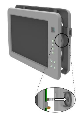
draw the cover close to the base so that the spring protecting against housing opening/removal fits correctly
