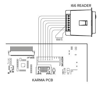
A connector (INSERITORE) is also available to connect a I66 reader: if necessary, wire it as indicated in the picture above and in its manual.
