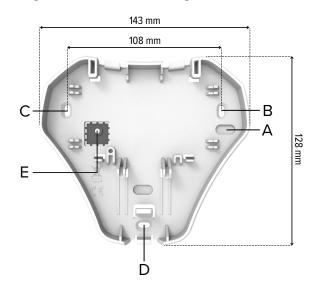
fix the base to the ceiling with screws and dowels using holes B, C, D
