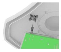
Verify that the spring protecting against housing opening is positioned correctly.
